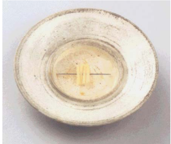
Mechanical Technology and Instruments of China. Fig. 16 A floating magnetic needle (from Zhongguo Gudai Keji Wenwu Zhan ).
